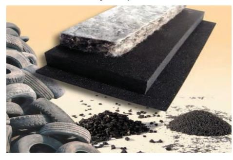
✓ Whereas most conventional thermoplastic powders do not meet the necessary requirements of this application such as not 'cracking' when flexed, a technically excellent product has been achieved using a powder to rubber crumb ratio as low as 10% - 15%. This is due to the excellent cohesive strength of Curabond along with a heat stable binding system.
